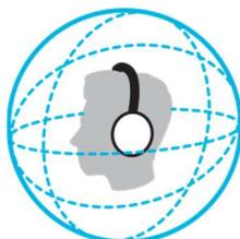
Ambisonics is the technology that uses a full-sphere surround sound technique to simulate spatial sound. Spherical harmonics is presented as the
